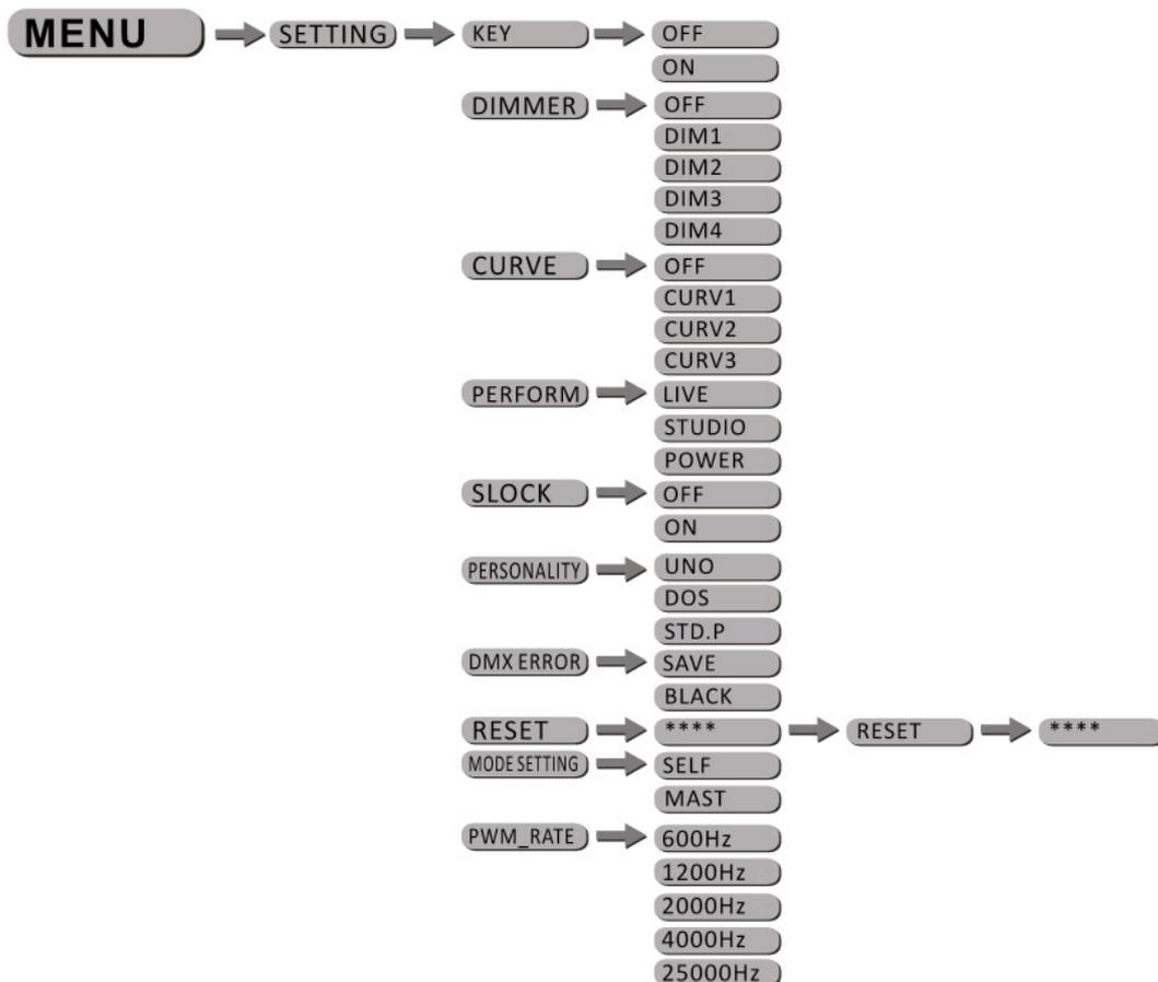
**SETTING** this menu allows the user to adjust key operation settings for this fixture. **KEY** select **ON** for automatic lock-out. Password to re-enter the display is **UP + DOWN + UP + DOWN**.
